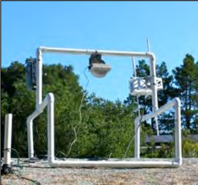
**Fig. 2: Roof mounted APs, POE cable carries power only**
